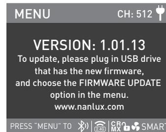
Rotate the "right knob" to VERSION, and press the "right knob" to check the current version.
