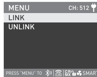
Rotate the "right knob" to LINK, and press the "right knob" to enter the next level menu.
