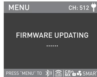
Connect a USB drive with the latest firmware file to the fixture, in the menu, rotate the "right knob" to FIRMWARE UPDATE, and press the "right knob" to enter.
