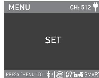
Rotate the "right knob" to select SMART, FULL SPEED, LOW SPEED and OFF, and press the "right knob" to set.
