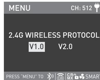
Rotate the "right knob" to WIRELESS PROTOCOL, and press the "right knob" to enter the corresponding next level menu.
