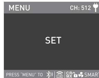
Rotate the "right knob" to select CCT 8bit, CCT 16bit or ULTIMATE DMX 8bit, and press the "right knob" to set.
