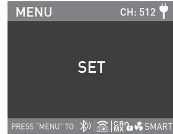
Rotate the "right knob" to select MAX OUTPUT or CONSTANT OUTPUT, and press the "right knob" to set.
